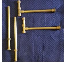
2. Start with the front legs. These come pre-assembled with the bottom collars set to support the metal tray 8" from the ground. The height of the collars can be adjusted using the set screw to suit desired design and space. If they are moved, the included wood block spacers will no longer be accurate.
