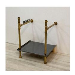
6. Install sink top and bracket according to the sink model. The stone sinks are counterbored on the underside to accept the top 3/8" of the front legs. The collars directly under the sinks do not support any weight. These can be adjusted up against the sink bottom when you are done with the final assembly.
