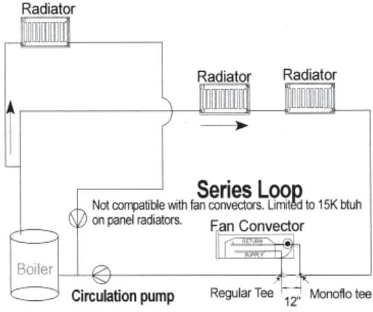
A single fan convector may be added to a series loop using monoflo tees.
