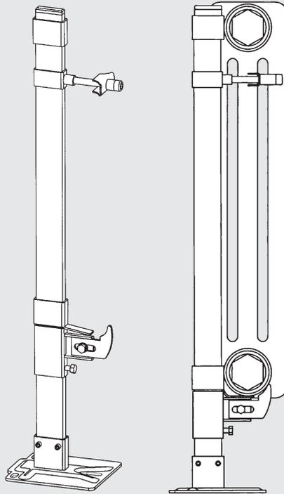
Complete system for free-standing radiators, from 2-6 column up to 1000mm height. Painted to RAL 9016.
