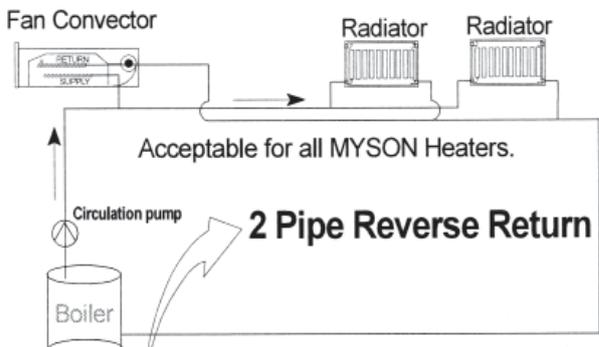
When mixing radiators of different head loss. i.e. fan convectors with radiators, balancing is often required to ensure proper flow through the fan convector.
