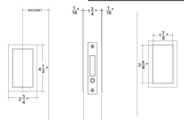
Minimum door thickness required is 1-3/4" when using with pocket lock
