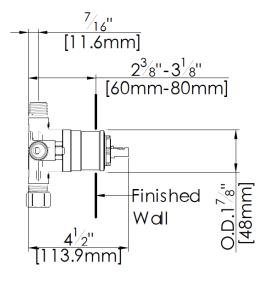
fluid Pressure Balancing Valve with Built-in 2 Way Diverter Model: F1002B F1002B-PEX F1002B-PEX-W
