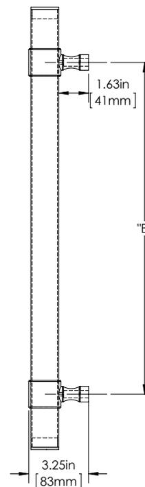
**Product Description:** 1 1/2" Tubular Round Grip with End Caps in Stainless Steel and Wrap Around Hourglass Mounts in Brass
