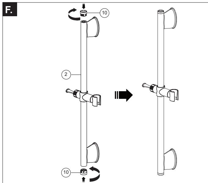
**F.** Once the adapters (9) and screws (8) are securely installed, screw the decorative end caps (10) into the ends of the slide bar (2).
