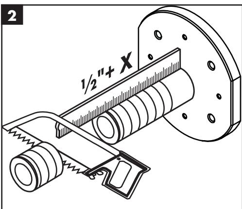
Mark the threaded nipple at a point  $1/2" + X$  from the back of the nipple assembly.
