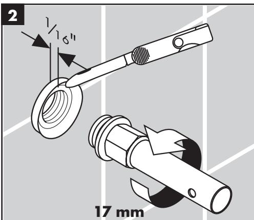
Cut the plaster shield so that it extends  $\frac{1}{16}$ " outside the surface of the finished wall.
