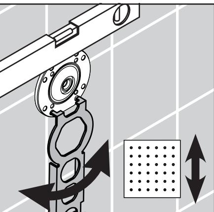
Use a level to make sure that the flat edges of the nipple flange are level.
