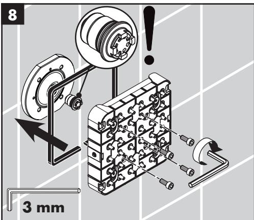
Press the flow restrictor into place in the nipple assembly.
