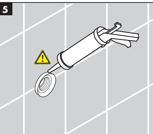
Seal the wall around the plaster shield using water-proof sealant.
