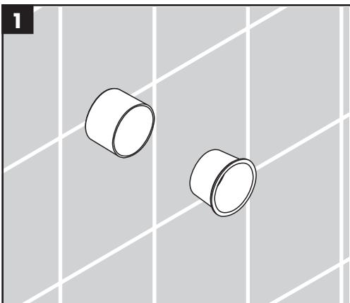
Remove the cover from the plaster shield.
