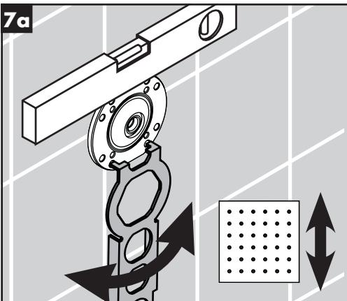
Use a level to make sure that the flat edges of the nipple flange are level.
