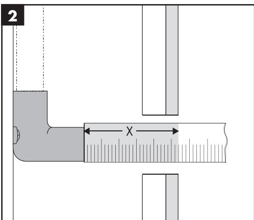
Measure the distance from the surface of the finished wall to the ell ("X").
