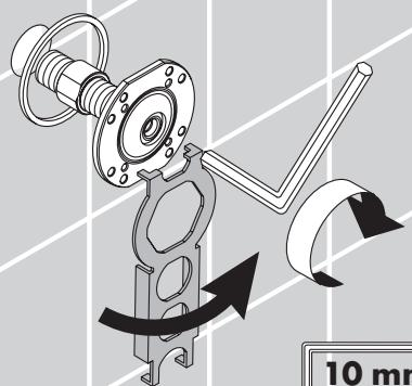
Install the shower module/adapter assembly using the service key and a 10 mm Allen wrench.
