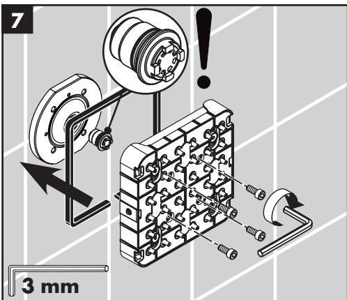
Press the flow restrictor into place in the nipple.
