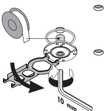
Wrap the threads on the nipple using plumber's tape.
