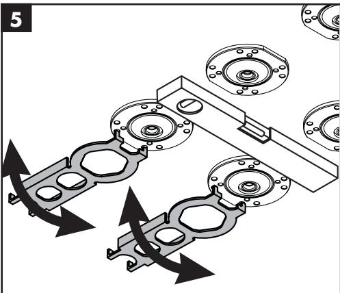
Use a level to make sure that the flat edges of the nipple flanges are level.
