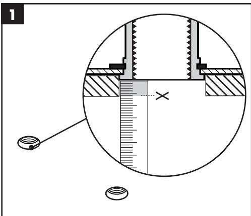
Measure the distance from the outside surface of the finished wall to the metal port on the rough ("X").
