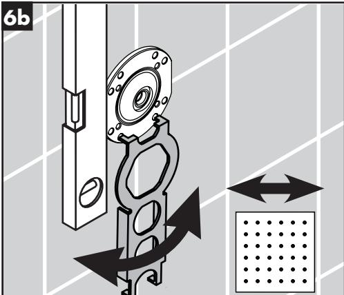
If you wish to be able to tilt the spray from side to side, the flat edges should be at the sides.
