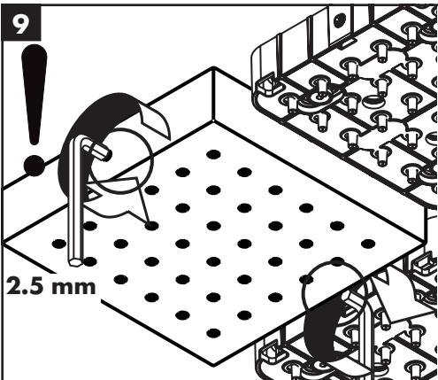
Secure the cover to the spray body by backing the screws out 3 complete rotations.
