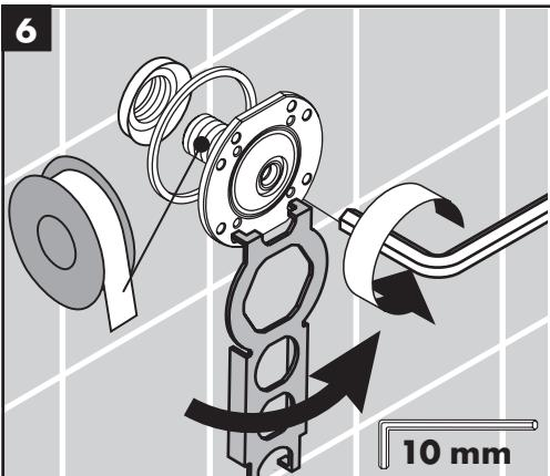
Wrap the threads on the nipple using plumber's tape.
